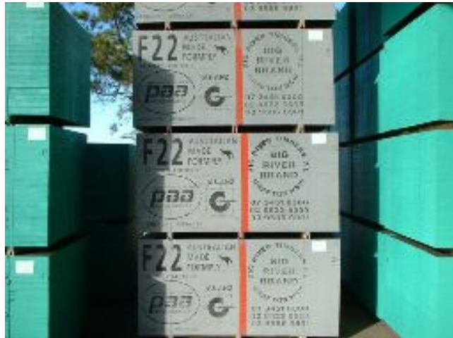
Certified formply is marked with an F value, along with both the EWPAAs and JAS-ANZ symbols.
